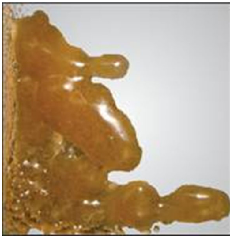
Figure 1 Solid obtained after spray drying autoclaved culture of B. subtilis LBBMA RI4914. Maltodextrin (100 g L -1 ) was added as a drying adjuvant.
