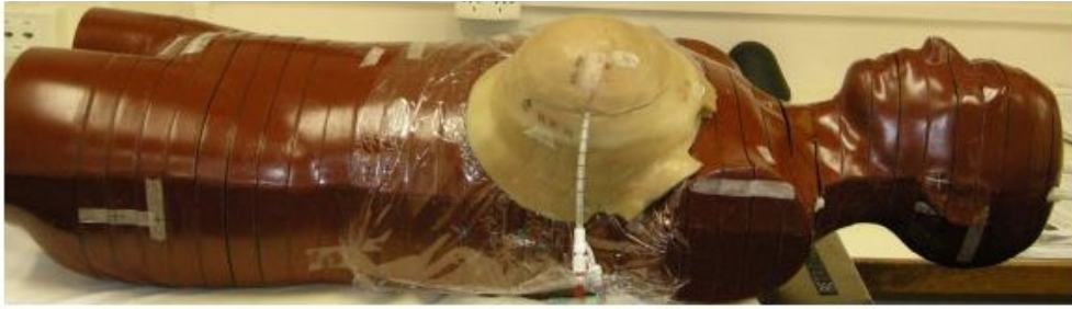
FIG. 1. The inflated balloon placed inside the breast tissue-equivalent phantom and attached to the Rando anthropomorphic phantom.
