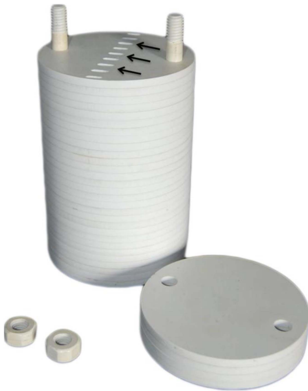
Figure 2. Clear polystyrene phantom employed in blood irradiation thermoluminescence dosimetry (TLD). Arrows show some cavities where TLD dosimeters were allocated. doi:10.1371/journal.pone.0065334.g002
