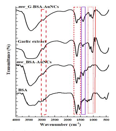
**Figure 2.** Fourier transform infrared (FTIR) spectra of *mw*\_G-BSA-AuNCs, pure garlic extract, BSA-gold nanoclusters (*mw*\_BSA-AuNCs) and BSA.
