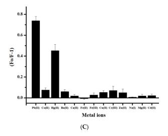
**Figure 5.** (A) Fluorescence spectra for the detection of Pb(II) ions by using mw\_BSA-AuNCs (concentration of Pb(II): (a) 0, (b) 1, (c) 2, (d) 4, (e) 6, (f) 8, (g) 10, (h) 16, and (i) 20 nM); (B) calibration curve for Pb(II) detection by using mw\_BSA-AuNCs; (C) fluorescence response of mw\_BSA-AuNCs for a 20 nM concentration of metal ions (n = 5).
