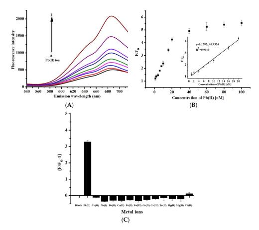
**Figure 4.** (**A**) Fluorescence spectra for the detection of Pb(II) ions by using  $mw\_G$ -BSA-AuNCs (concentration of Pb(II): (**a**) 0 nM, (**b**)1 nM, (**c**) 2 nM, (**d**) 4 nM, (**e**) 6 nM, (**f**) 8 nM, (**g**) 10 nM, (**h**) 16 nM, and (**i**) 20 nM); (**B**) calibration curve for Pb(II) detection by using  $mw\_G$ -BSA-AuNCs; (**C**) fluorescence response of  $mw\_G$ -BSA-AuNCs for a 20 nM concentration of common metal ions (n = 5).
