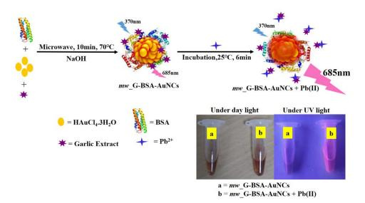
**Figure 1.** Scheme for the "off-on" method of bovine serum albumin (BSA)-gold nanoclusters with garlic extract modifications (*mw*\_G-BSA-AuNCs).
