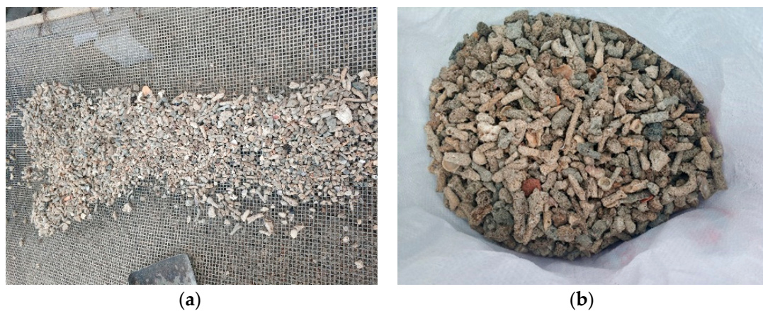
Figure 1. Coral aggregates for test: (a) broken coral; and (b) coral aggregates.
