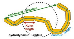
**Figure 6.** Scheme of polymer structural parameters. The cartoon sketches the main structural parameters identified in the experimental work, namely the end-to-end distance (green solid arrow), the contour length (blue solid curve), the hydrodynamic radius (black dashed circle), and the Kuhn length (red solid arrow).
