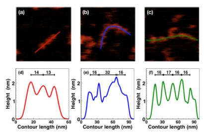
Figure 3. (a–c): Zoom of three regions of 100 nm  $\times$  100 nm size, selected from dashed squares in Figure 1. The elongation axis, or contour profile, of polymers is marked with colored solid curves. (d–f): height profiles along the contour length of polymers displayed in (a–c) respectively. The solid bars within each panel report the pitches between two peaks in the height profile; the numbers above each bar are the length in nanometres.
