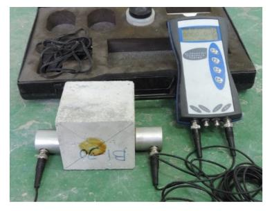
Figure 3. The ultrasonic pulse velocity test device.
