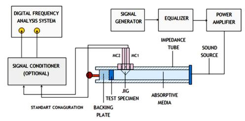
**Figure 4.** Configuration of impedance tube and experimental setup for acoustic transmission according to ASTM E1050.
