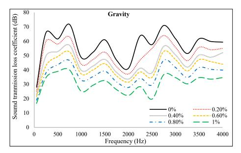
Figure 13. Sound transmission loss coefficient of PAFRC mixtures.
