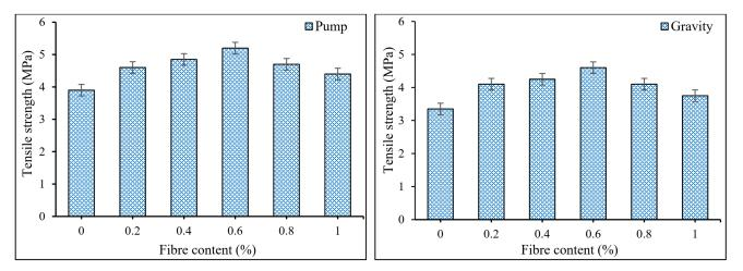
Figure 6. Influences of PP fibers on the tensile strength of PAFRC mixtures.
