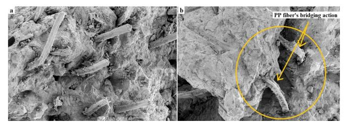
Figure 7. (a) Distribution of PP fibers in the matrix and (b) the fiber's bridging action.
