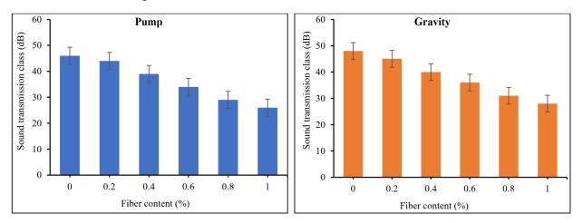
Figure 14. Sound transmission class PAFRC mixtures.
