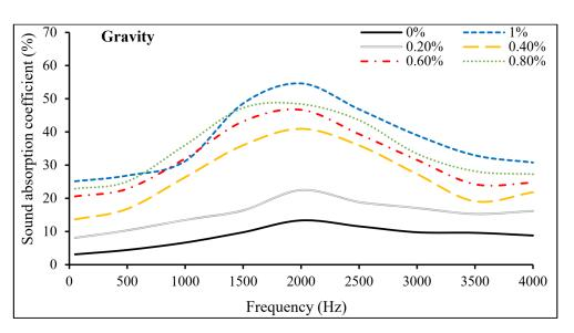
Figure 10. The sound absorption coefficient of PAFRC mixtures.
