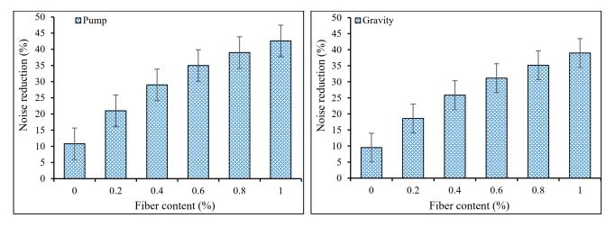
Figure 11. Noise reduction coefficients of PAFRC mixtures.
