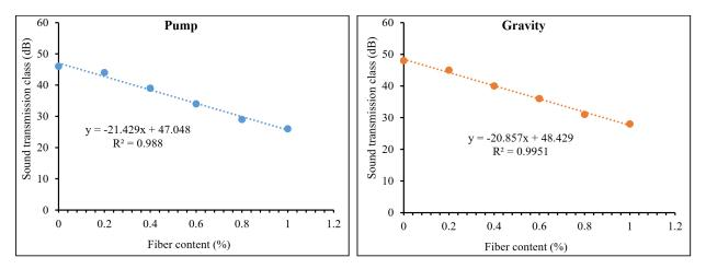
Figure 15. Correlations between the sound transmission class and fiber dosages of PAFRC mixtures.
