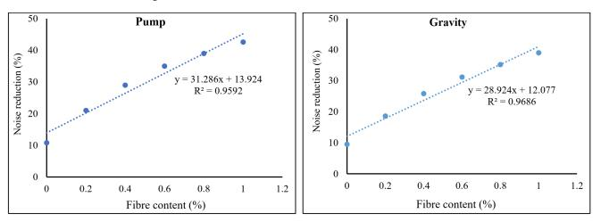
Figure 12. Correlations between noise reduction and fiber content of PAFRC mixes.
