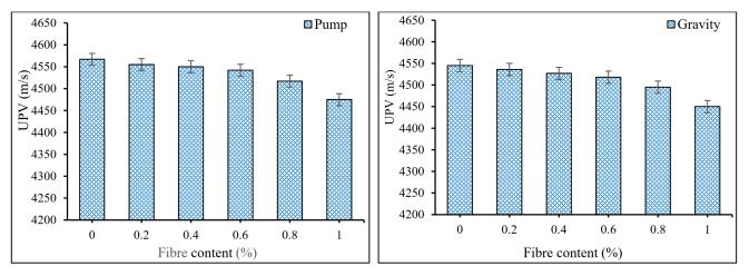
Figure 8. The variation in UPV values of PAFRC mixtures with different fiber contents.
