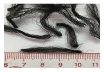
Figure 1. Size and shape of PP fibers used.
