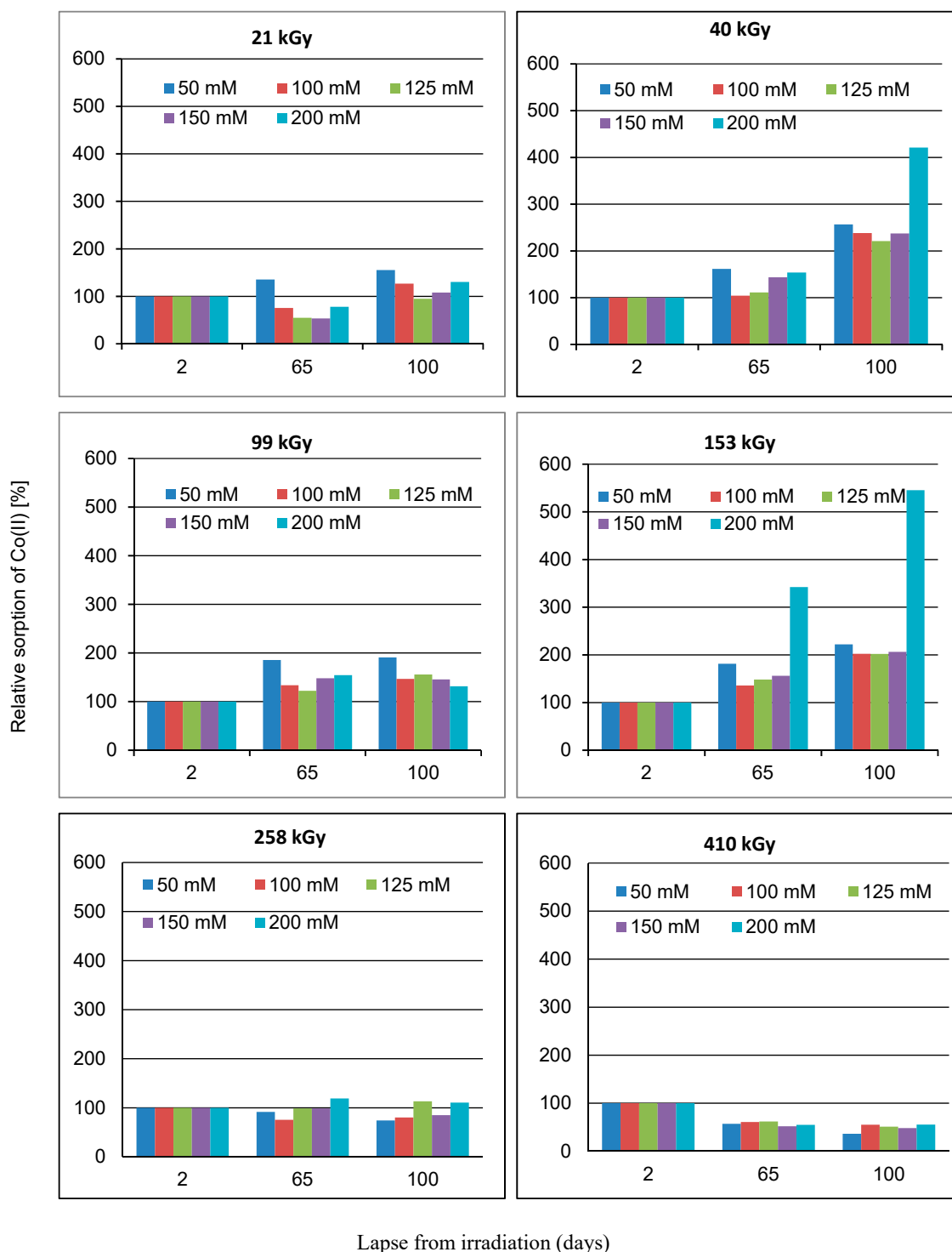
Figure 6. Relative time variation of Co(II) sorption on the wool compared with sorption for 2-day's lapse from the exposure.
