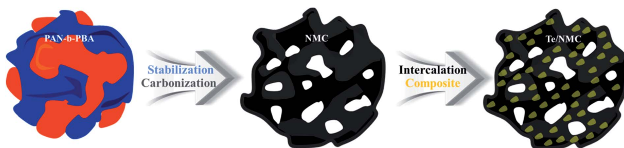
Fig. 1 Preparation method of the tellurium/nitrogen-doped mesoporous carbon composite material.
