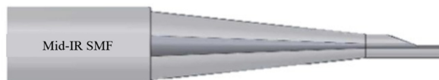
Figure 1. The scheme of light coupling from a mid-IR SMF to a DSCF through a tapered SCF region.
