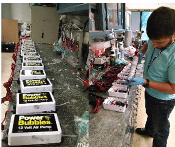
Figure 1. Sealing and preparing recirculation pumps. Sealing recirculation pumps for field deployment.
