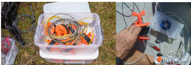
Figure 4. Modified well caps showing gas recirculation lines. This figure shows well caps modified with gas inlet and return lines.
