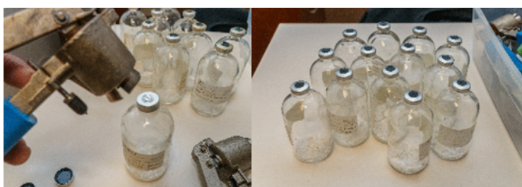
Figure 2. NaOH traps prepared for field deployment. 120 ml serum bottles with NaOH trap added and crimp sealed.
