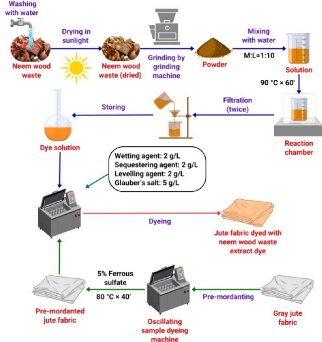
Figure 16. Schematic presentation of the dye extractions and jute fabric dyeing with neem wood waste powder. Reproduced with permission from Mia et al. 97 Copyright 2024, Elsevier Science Ltd.
