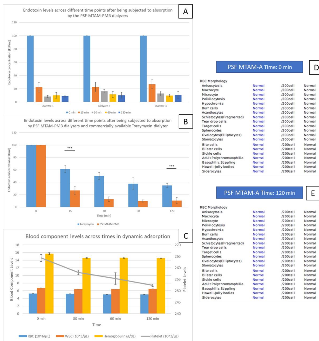
Figure 8. Endotoxin levels across different time points of three samples of the PSF MTAM-A-PMB based hemoperfusion unit (A); n = 3 for each sample point). Comparison between the performance of the commercially available Toraymyxin endotoxin removal system versus the PSF MTAM-A-PMB based hemoperfusion unit (internally conducted). (B) The performance of the PSF MTAM-A-PMB hemoperfusion system achieved a rapid removal of up to 73.18%, while the commercial latter registered a value of 38.78%. The total removal capacity of the PSF MTAM-A-PMB hemoperfusion system was 89.43%, compared to the commercial latter, which was 65.03%. Changes in blood components across time (C). Pathological analysis conducted at Union Clinical Laboratory (UCL) of the red blood cell morphology per and post absorption (D,E). Statistical definition: p -value \leq 0.05 (***)
