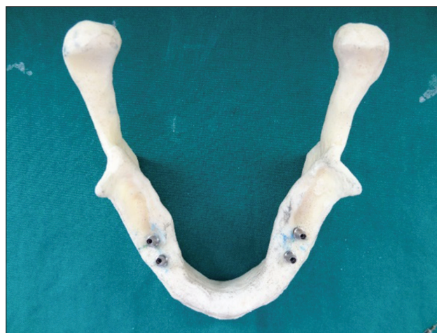
Figure 1: Polyurethane mandibular model with implants and abutments
