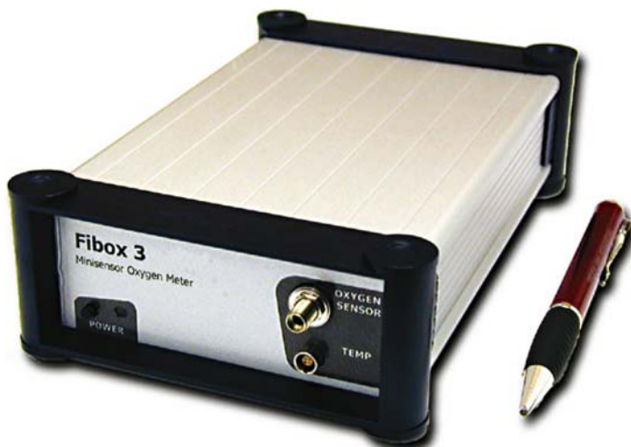
Fig. 4.47 Single channel instrument for the measurement of oxygen using an optode (with permission and by courtesy of Presens Sensing GmbH, Germany)
