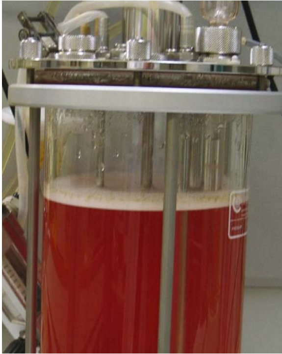
Fig. 4.27 5–10 mm foam layer at the medium surface (cell line: CHO-easyC – CHO-K1 derived line, Cell Culture Technologies GmbH, Zürich, Switzerland; CHO-master HP-1 medium; aerated with a ceramic micro sparger Fig. 4.18)
