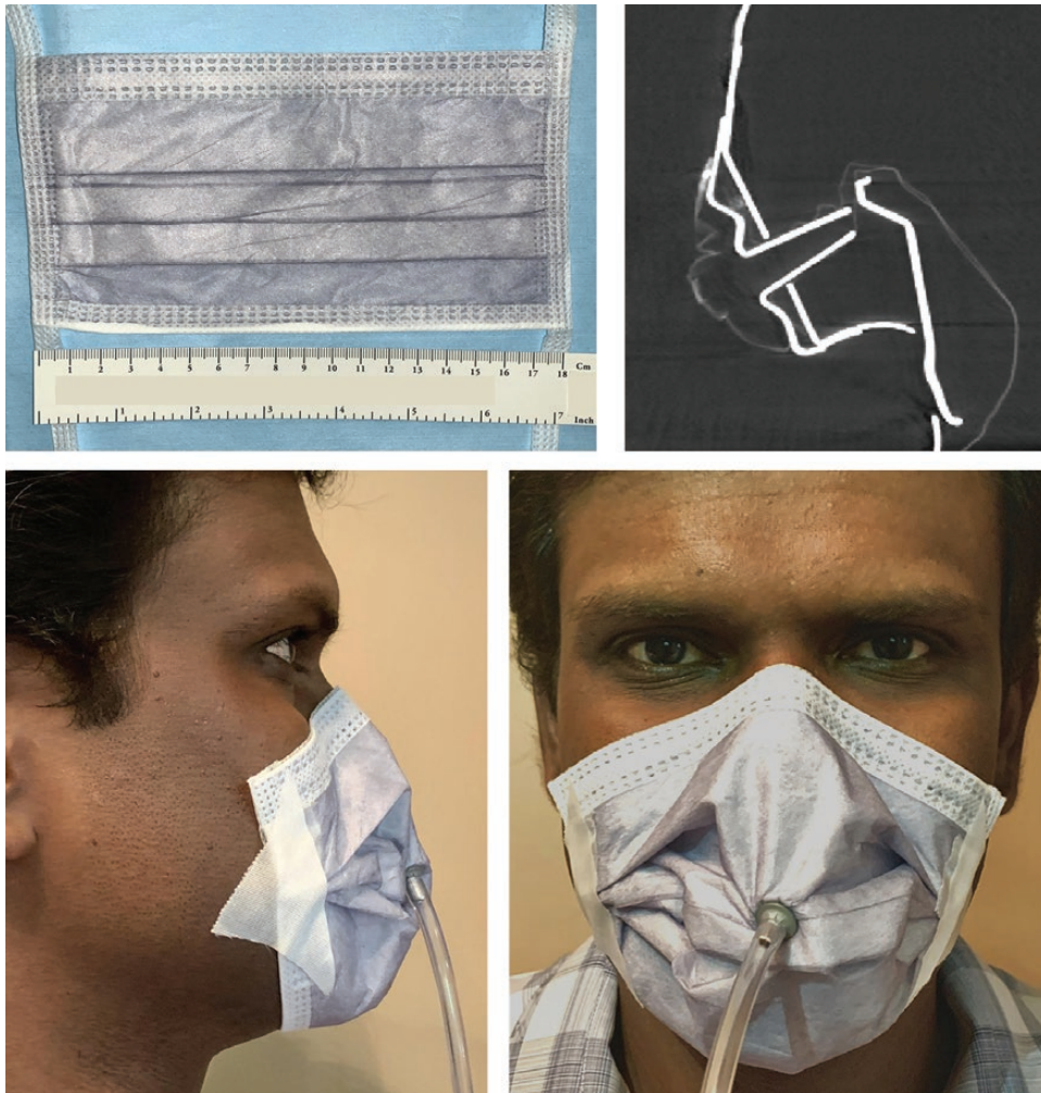
Figure 1. Sealed surgical masks used in this study. Top left panel: photograph of surgical mask used in the study. Top right panel: illustration of sealed surgical mask donned on a manikin using a sagittal reconstruction computed tomography image. Bottom panels: sealed surgical mask with sampling probe and hose during a fit test.
