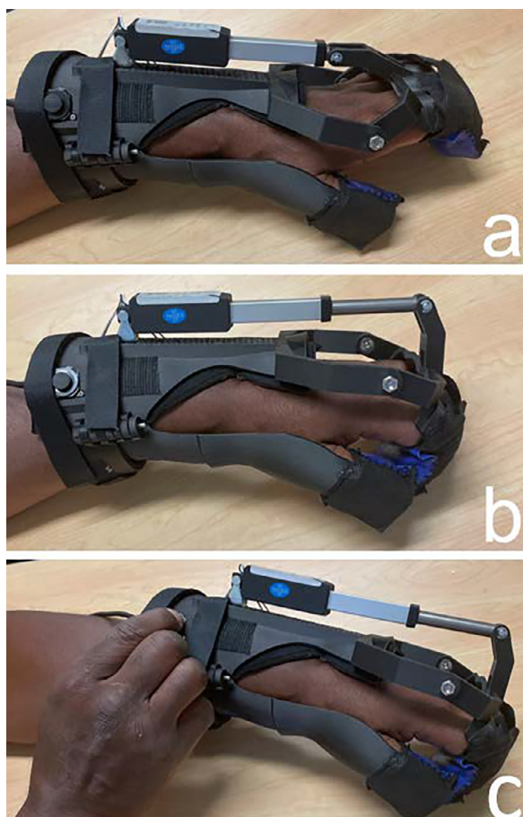
Fig 4 Participant NS7 wearing the 3D printed NuroSleeve design (a) in the hand open position, (b) in the closed position, (c) and triggering finger flexion by using an mounted joystick controller with the unaffected hand.
