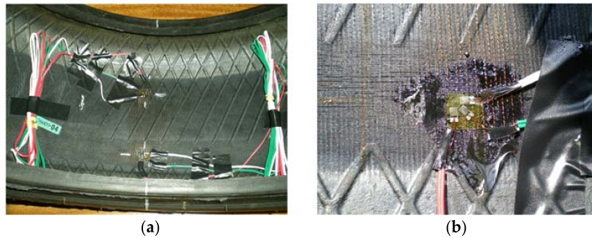
Figure 4. (a) Strain gauges’ setup; (b) Multi-axial gage example.
