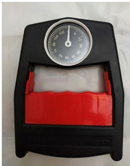
Figure 2. Handheld dynamometer used to measure the hand-grip strength.
