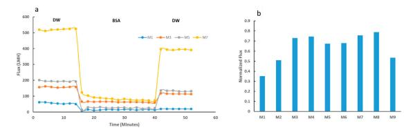
**Figure 10.** Fouling tests using BSA solution for selected membranes. (a) The initial deionized water (DW) flux was measured before bovine serum albumin (BSA) filtration and then final DW flux was measured for each selected membrane. (b) Normalized flux data for selected PES membranes, calculated as a ratio of final DW flux to initial DW flux.
