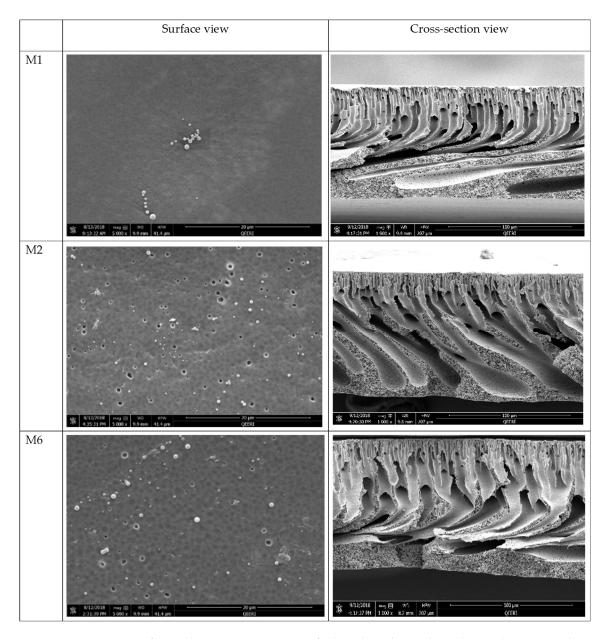
**Figure 4.** FESEM surface and cross-section images of selected synthesized membranes (M1, M2, and M6).
