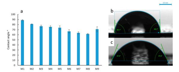
**Figure 6.** Average water contact angle readings for the synthesized PES membranes (a), sample photographs of water droplets with angle measurements for selected samples of M1 (b) and M8 (c). Each bar represents the mean  $\pm$  SD of five independent readings.
