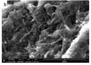
**Figure 1.** Field emission scanning electron microscopy (FESEM) images for multiwalled carbon nanotubes (MWCNT) (a), oxidized multiwalled carbon nanotubes (OMWCNT) (b).
