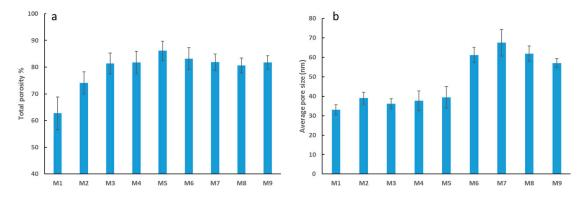
**Figure 5.** Total porosity of fabricated PES membranes (a), and average pore size of fabricated PES membranes (b). Each bar represents the mean  $\pm$  SD (standard deviation) of three independent readings.
