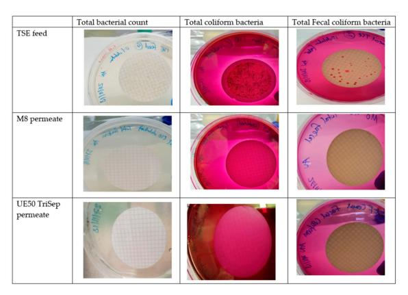
**Figure 16.** Images of agar plates with cellulose discs used for filtering either TSE feed or permeates of TSE filtration, using M8 and commercial UE50 TriSep membranes.
