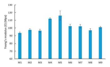
**Figure 9.** Average Young's modulus values for synthesized PES membranes. Each bar represents the mean  $\pm$  SD of three independent readings.
