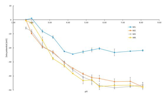
**Figure 7.** pH scans for selected fabricated PES membranes displaying zeta potential readings. Each bar represents the mean  $\pm$  SD of three independent readings.
