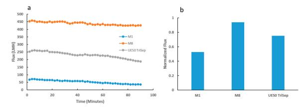
**Figure 14.** Flux readings for synthesized and UE50 TriSep membranes over a prolonged period of bacterial suspension filtration (a). Normalized flux data for each of the three membrane samples (b).
