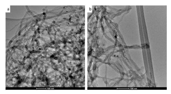
**Figure 2.** Transmission electron microscopy (TEM) images of multiwalled carbon nanotubes (MWCNT) (a) and oxidized multiwalled carbon nanotubes (OMWCNT) (b).
