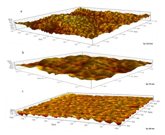
**Figure 8.** 3D AFM surface images for M1 (a); M7 (b); and M8 (c) samples. Mean surface roughness (Sa) values are indicated.
