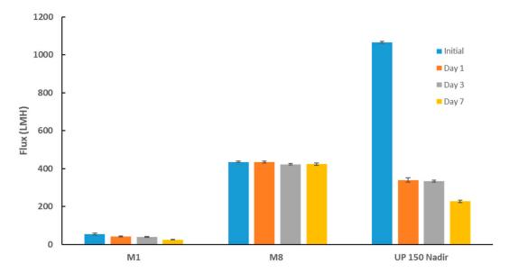
**Figure 15.** Membrane flux before incubation with bacterial suspensions and post incubation at different time points. Each bar represents the mean  $\pm$  SD of three independent readings.
