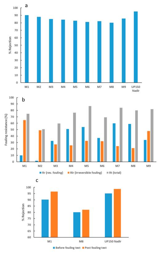
**Figure 11.** Rejection and fouling data for fabricated PES membranes. (a) BSA rejection values, (b) different types of membranes fouling derived from BSA solution filtration tests, and (c) BSA rejection values for M1, M8, and UP150 Nadir commercial membrane before and after filtration with *E. coli* suspension.
