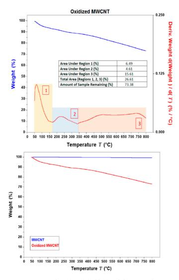
**Figure 3.** (a) Thermo-gravimetric analysis (TGA) (in blue) and derivative thermo-gravimetric analysis (DTGA) (in red) thermograms for OMWCNT. The area under the different segments of the graph are quantified in the insert. (b) Overlay of the TGA thermograms for both MWCNT (in blue) and OMWCNT (in red).
