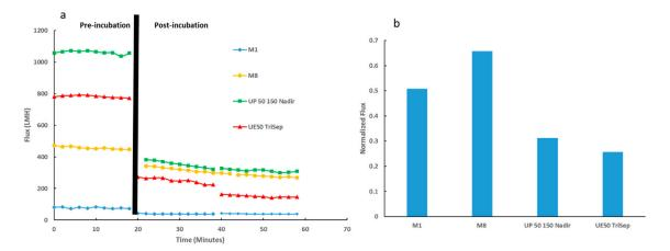
**Figure 13.** Membrane performance testing for PES-synthesized membranes and commercial membranes. (a) Flux readings for membranes before and after incubation with *E. coli* suspension (denoted by black line). (b) Normalized flux data for membranes tested.
