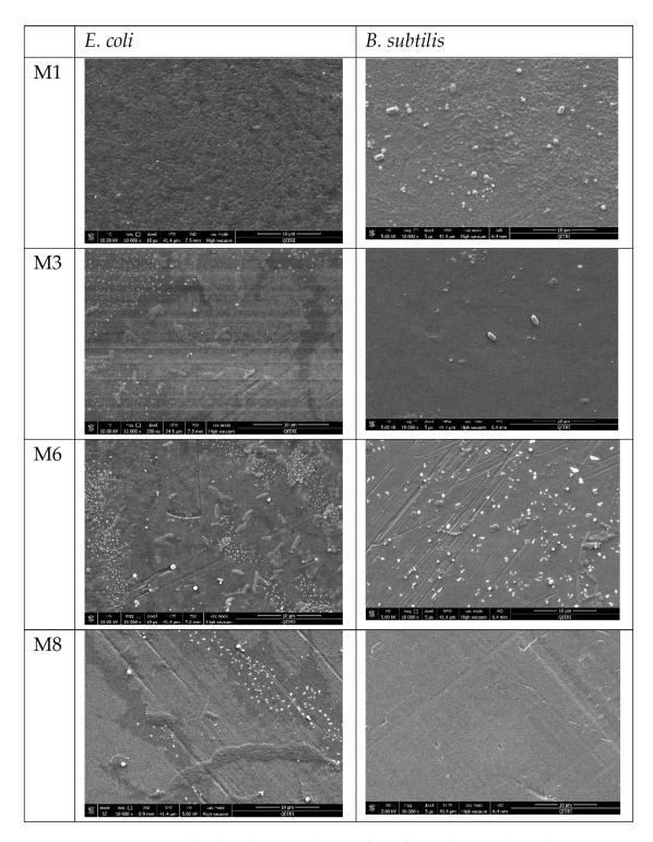
**Figure 12.** FESEM images for selected PES membrane surfaces after incubation with *E. coli* suspension (**left side panel**) and with *B. subtilis* suspension (**right side panel**).
