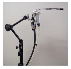
**Figure 2.** Fixation device comprising a commercially available light stand and a multi-jointed arm. This system enables arbitrary positioning.
