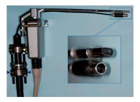
**Figure 1.** The endoscope was 5.4 mm in diameter. Two 1/10 inch micro charge-coupled device cameras are mounted into the tip of the endoscope. The lens of the pattern projection system, which is mounted in the system's tip. A latticework pattern is placed on the bottom of the endoscope (arrow).
