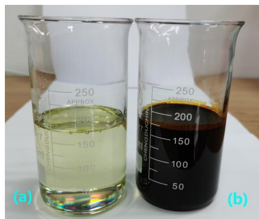
Figure 12. Epoxy resin used in this study: (a) epoxy oligomer and (b) hardener.
