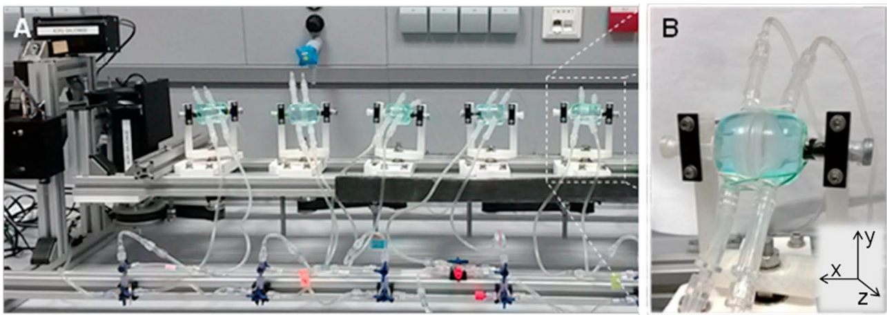
Fig. 10 Eye movement system (A); vitreous models (B) developed by Stein and colleagues. Reproduced with permission from [72]
