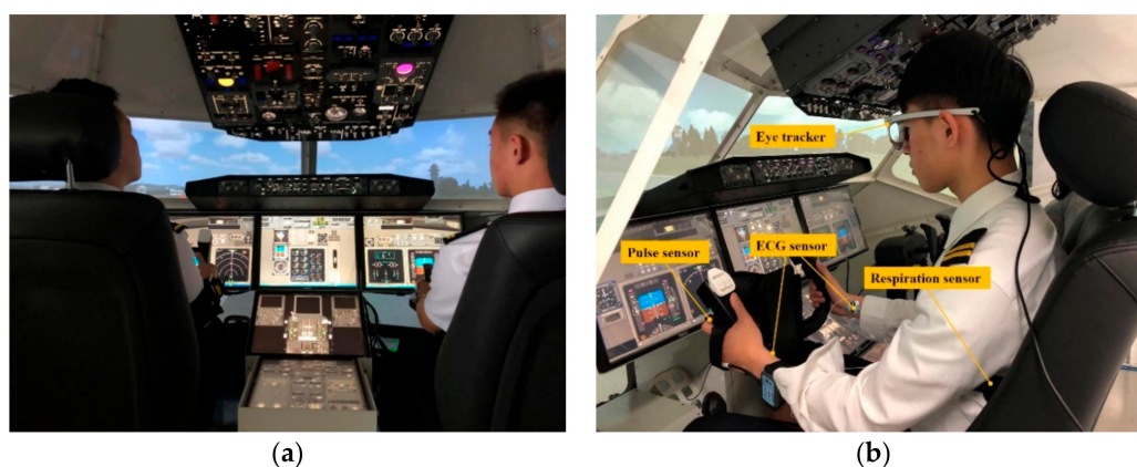
Figure 5. Experiment scenes of flight simulation. (a) Flight simulation experimental platform. (b) Flight personnel wearing physiological monitoring sensors during the experiment.
