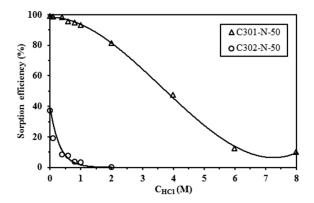
**Figure 1.** Effect of HCl concentration on the sorption of Pb(II) using Cyanex 301 and Cyanex 302 encapsulated in alginate mononuclear capsules (sorbent dosage, SD: 2 g·L<sup>-1</sup>; contact time: 4 days; T: 20 °C;  $C_0$ : 50 mg·Pb·L<sup>-1</sup>; extractant concentration in kerosene: 50% v/v; agitation speed, v: 150 rpm).
