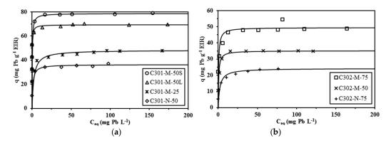
**Figure 2.** Pb(II) sorption isotherms using Cyanex 301 (a) and Cyanex 302 (b) encapsulated in alginate capsules (M: matrix-type capsules; N: mononuclear capsules) (solid lines: modeling of sorption isotherms with the Langmuir equation and coefficients reported in Table 2) ( $C_{HCI}$ : 0.1 M; contact time: 4 days; T: 20 °C; v: 150 rpm).
