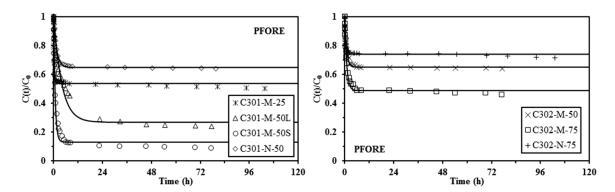
**Figure 4.** Pb(II) uptake kinetics using Cyanex 301 and Cyanex 302 immobilized in alginate capsules (M: matrix-type capsule; N: mononuclear capsule) (solid lines: modeling of uptake kinetics with the PFORE - and coefficients reported in Table 4) ( $C_0$ : 170 mg·Pb·L<sup>-1</sup>; SD: 2 g·L<sup>-1</sup>;  $C_{HCl}$ : 0.1 M; v: 150 rpm; T: 20 °C).
