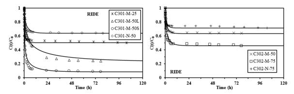
**Figure 3.** Pb(II) uptake kinetics using Cyanex 301 and Cyanex 302 immobilized in alginate capsules (M: matrix-type capsule; N: mononuclear capsule) (solid lines: modeling of uptake kinetics with the RIDE—Crank equation—and coefficients reported in Table 3) ( $C_0$ : 170 mg·Pb·L<sup>-1</sup>; SD: 2 g·L<sup>-1</sup>;  $C_{HCI}$ : 0.1 M; v: 150 rpm; T: 20 °C).
