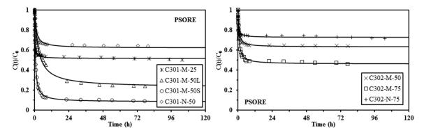
**Figure 5.** Pb(II) uptake kinetics using Cyanex 301 and Cyanex 302 immobilized in alginate capsules (M: matrix-type capsule; N: mononuclear capsule) (solid lines: modeling of uptake kinetics with the PSORE - and coefficients reported in Table 4) ( $C_0$ : 170 mg·Pb·L<sup>-1</sup>; SD: 2 g·L<sup>-1</sup>;  $C_{HCl}$ : 0.1 M; v: 150 rpm; T: 20 °C).
