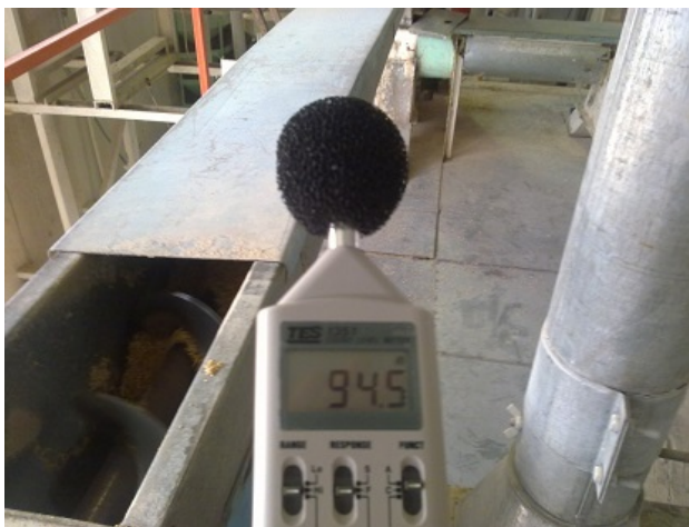
Fig. 1 Moment of measuring noise in production hall
