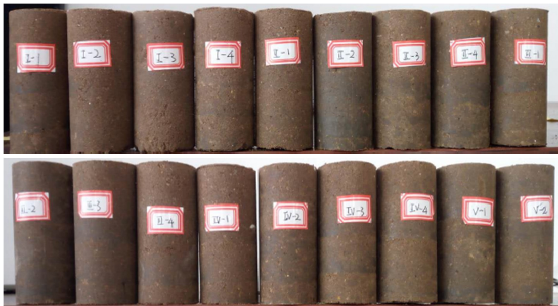
Figure 2. Prepared cement improved aeolian sand (CIAS) sample.
