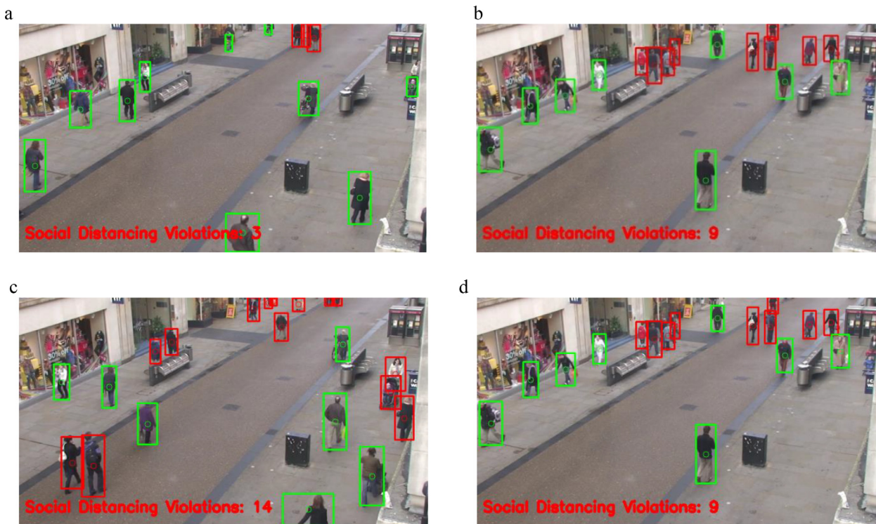
Fig. 6. (a) - (d) shows the output of the Deep Learning Six feet Apart analysis at different instances of the processed video where the text on the left-hand side indicates the number of violations that have happened at each second of the video at that particular instance.
