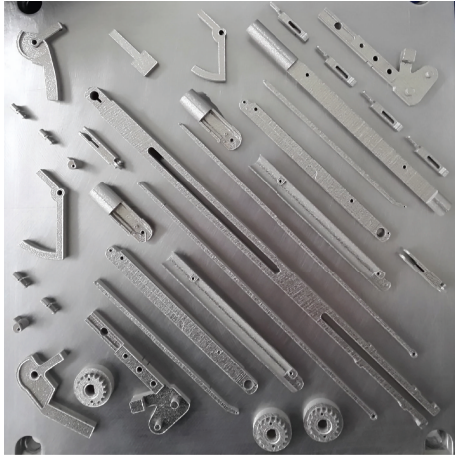
FIGURE 10: The 3D output plate holding the different components.
