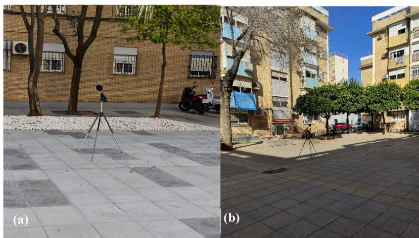
Fig. 3. (a) Measurements in La Debla Plaza, Receiver 12; (b) Behind the dwelling whose acoustic insulation has been studied, Receiver 11. For its acoustics data see Section 5.2. Tables 5 and 6.
