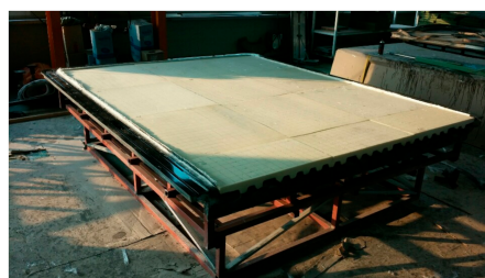
Figure 16. Application of foam core for sandwich composite structure.
