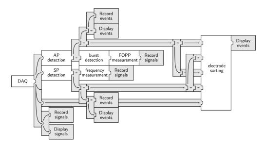
Figure 11. Multimed processing architecture for pancreatic islet screening.
