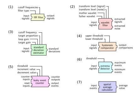
**Figure 5.** Processing units from Multimed's module library. Square inputs/outputs represent event connections and round inputs/outputs represent signal stream connections. The numbering of the modules refers to that of both Table 1 and the current section.
