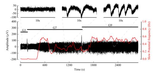
**Figure 12.** Raw signal (black) and Slow Potential (SPs) frequency measurements (red) on a mouse islet culture, using a Qwane MEA with microfluidic features. Zoom on three representative samples of the measured biosignal to provide a clearer illustration of changes in measured activity. Experimental protocol is described with the "G3", "G7", and "G9" labels, indicating changes in glucose concentrations in mM/L.
