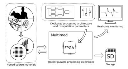
**Figure 1.** Multimed and its interfaces. From left to right: User parameters are fed into the system, which is connected to the measured and/or stimulated cell culture. The board then processes the data using a Field Programmable Gate Array (FPGA), which displays measurements on an external screen and records unprocessed and processed data to SD cards.
