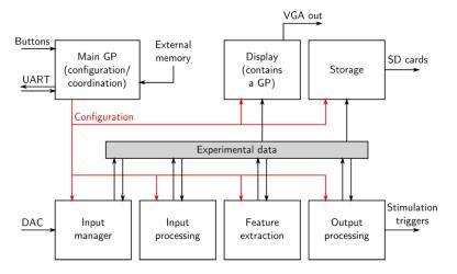
**Figure 4.** High-level data flow of Multimed. The generic processor (GP) is separate from the data processing chain and only helps as a means of communicating and configuring. All of the digital processing modules feed off the same data bus (Experimental data), minimizing dependencies and facilitating complex connections.
