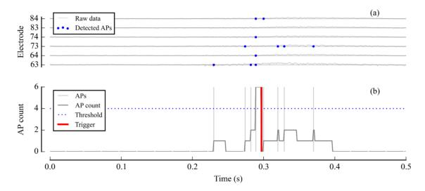
**Figure 15.** A stimulation command triggered by synchronized spiking activity in a neuron culture. The trigger was set off when more than four APs were detected across six selected channels in a 25 ms time window. (a) Unprocessed data on one of the channels of interest; (b) AP detection on the six channels of interest and, (c) Illustration of synchronization detection: AP count and related trigger.
