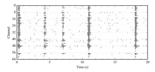
**Figure 9.** Raster plot of real-time neural AP detection on a patterned culture, recorded on a 60-electrode MEA. In this reading, the average burst contained 11 APs per electrode. The experimenter validated detected events offline.
