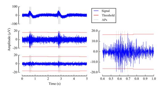
**Figure 10.** Detail of real-time AP detection on a neuron culture using an adaptive threshold and Haar wavelet filtering. Signals shown are: A: raw signal and AP detection; B: 4th wavelet transform level on which detection was performed, detection threshold, AP detection; and, C: 1st wavelet transform level, on which the detection threshold was computed, detection threshold, and AP detection. The experimenter visually validated detected events.
