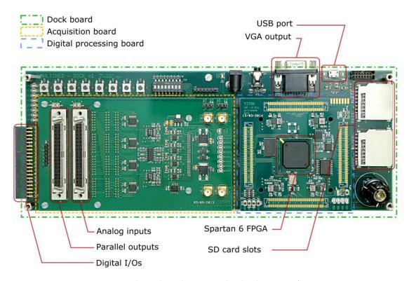
Figure 2. The Multimed system and its hardware interfaces.
