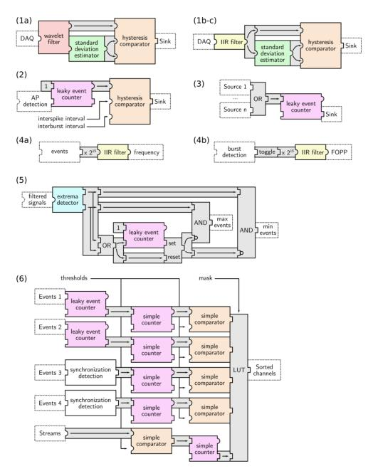
**Figure 6.** Combinations of processing units generate more complex functions. Numbering refers to that of Table 2. (1a): Adaptive wavelet AP detection; (1b-c): Adaptive AP-Local Field Potentials (LFP) detection; (2): burst detection/AP cleaning; (3): Synchronization detection; (4a): Event frequency measurement; (4b): Burst Fraction of Plateau Phase (FOPP) measurement; (5): Extremum detection; and, (6): Electrode sorting. Blocks in dotted lines indicate connection context.
