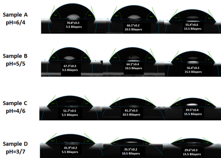
Figure 11. Contact angle measurement of thin film gradients at various pH combinations.
