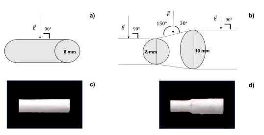
**Figure 1.** (a) Cylindrical mandrel surface perpendicular to electric field; (b) asymmetrical mandrel junction not perpendicular to electric field; (c) polymeric cylindrical scaffold; (d) polymeric asymmetrical scaffold.
