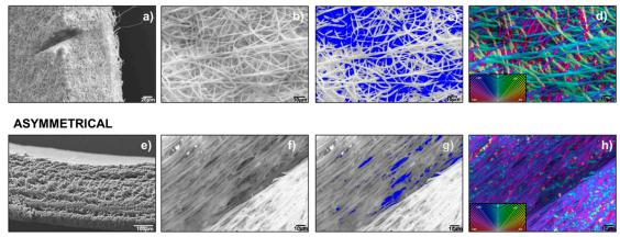
**Figure 2.** Images of cylindrical scaffold: (**a**) SEM-scaffold thickness, (**b**) SEM- scaffold inner surface, (**c**) Imagej segmentation of SEM image, (**d**) Imagej orientation of SEM image (**a**). Images of asymmetrical scaffold: (**e**) SEM-8 mm diameter scaffold thickness, (**f**) scaffold inner surface, (**g**) Imagej segmentation of SEM image, (**h**) Imagej orientation of SEM image (**f**).
