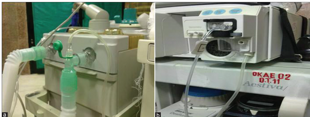
Figure 1: Special connector for return of sampling gas used. (a) One end of the connector attached to the expiratory limb of breathing circuit. (b) Second end of connector attached to the exhaust of respiratory gas monitors (RGM)
