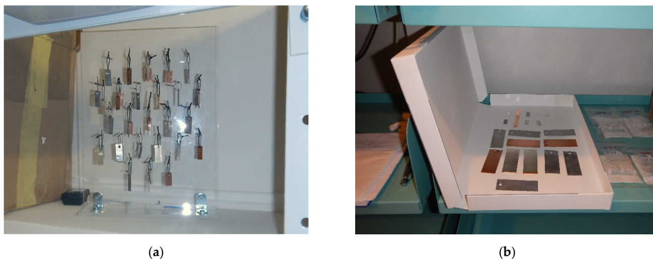
Figure 1. Corrosion coupons: (a) fixed to stand at location 13; (b) placed in modern archive box at location 10.
