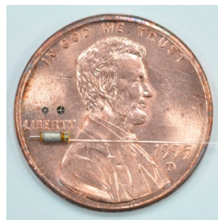
Figure 13. A 1 mm diameter micromotor with an optical encoder.
