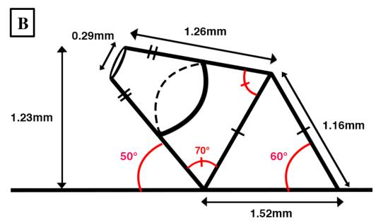
**Fig 1. Image of three-dimensionally printed spring with angled bidirectional surface features.** (A) Direction of features is indicated by the arrows. One of the surface hooks is isolated by a box. Scale bar is 5 mm. (B) Zoomed in side view schematic of isolated surface feature and corresponding dimensions.
