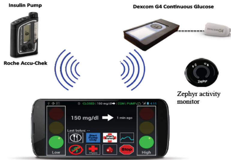
Figure 2. Portable system used in more recent studies reported in Cameron et al. [43,44].
