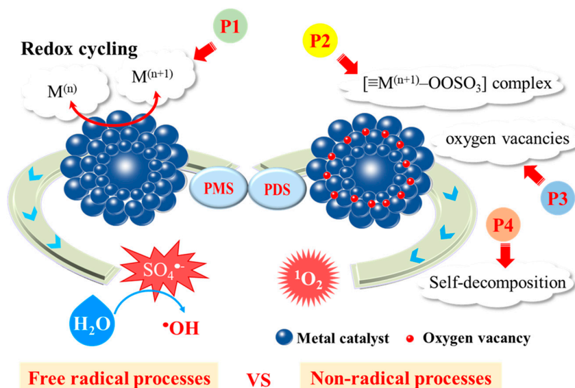
Figure 5. Schematic illustration of pathways of PMS/PDS activation in metal-catalyzed heterogeneous systems. P1: redox cycling; P2: formation of metal-PMS/PDS complex; P3: generation of oxygen vacancies; P4: PMS/PDS self-decomposition.
