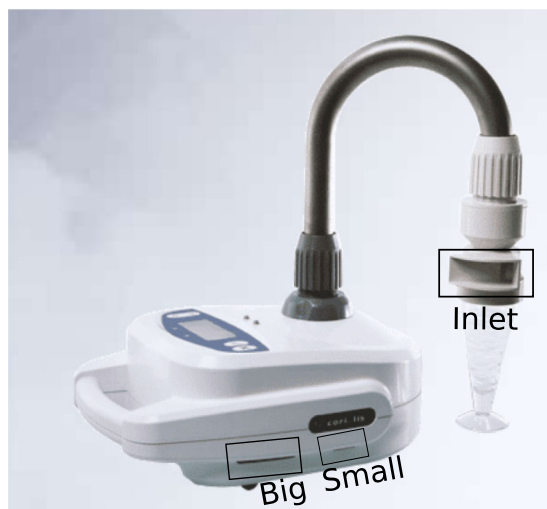
Fig. 2 Simplified intake model from “Coriolis Micro” air sampler by “Bertin Technologies”
