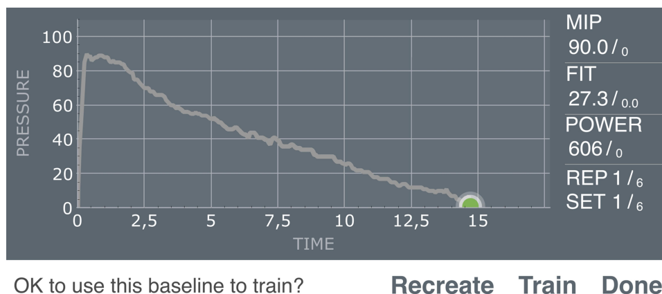
Figure 3 Graphic presentation of a sustained maximal inspiratory effort performed using the PrO2 device and software. In this example, the user achieved a MIP of 90 cmH 2 O, a SMIP of 606 PTU reflecting the area under the pressure-time curve. The entire maneuver lasted 15 seconds.
