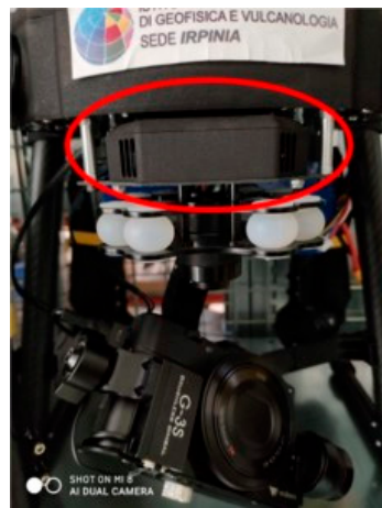
Figure 4. GNSS module integration on a drone.
