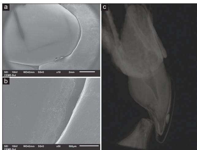
Figure 6: (a) Scanning electron microscope images of ceramic veneer bonded to maxillary right central incisor after 123 months of clinical service. (b) Tooth-resin composite-ceramic interface had no wear, gaps, or any sign of degradation, with a smooth transition between substrates (a) x10; (b) x50. (c) Cone-beam computed tomography image of same tooth showing excellent adaptation of ceramic veneer
