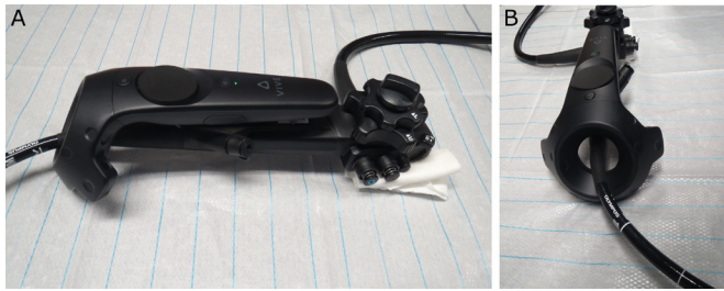
Figure 1 Virtual reality-controller mounted on a regular gastroscope.
