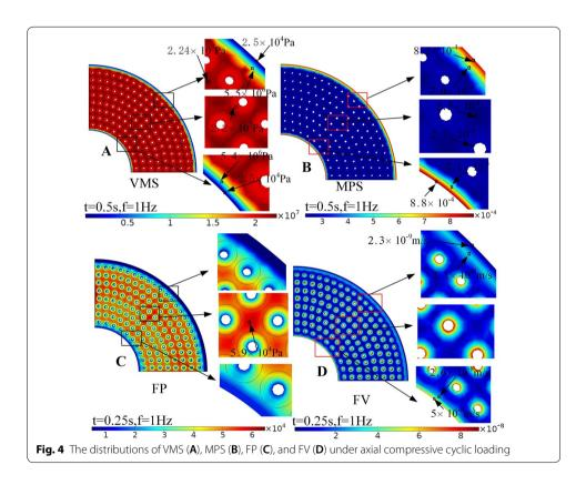
generally higher than that in other locations (Fig. 4A). The maximum VMS at periosteum ( $5.5 \times 10^6$  Pa) and endosteum ( $2.5 \times 10^5$  Pa) had minimum values among all functional units (Fig. 4A), while the maximum MPS ( $8.4 \times 10^{-4}$  and  $8.8 \times 10^{-4}$ ) was
