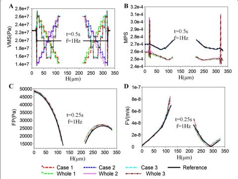
**Fig. 7** Effects of different E in each osteon lamella on mesoscale model. The maximum responses of VMS (**A**), MPS (**B**), FP (**C**), and FV (**D**) along the line H for the whole models (Whole 1, 2, and 3) and the mesoscale models (Cases 1, 2, and 3)
