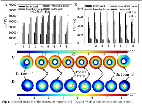
Region 8 (Fig. 1e). The distributions of FP (C) and FV (D) of Osteon 1-Osteon 8 (Fig. 1e)
