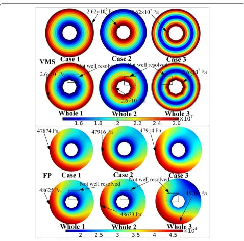
**Fig. 6** The distributions of maximum VMS and FP over the selected osteon. The whole model (Whole 1, 2, and 3) and the mesoscale models (Cases 1, 2, and 3) are compared
