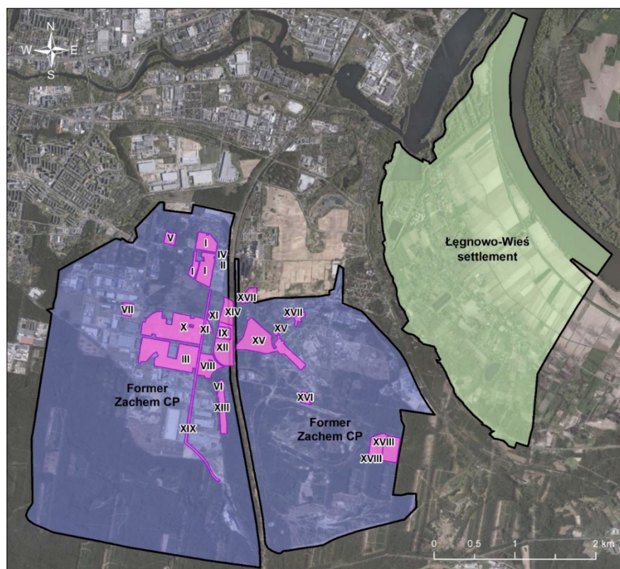
Figure 2. Location of the main contamination sources in the former ZACHEM CP area by BRDEP, based on Czop et al. [37]; I: dye plant, II: dye waste pit, III: monomer complex installation, IV: cold control unit, V: manufacturing of polyester polyols and polyurethane systems, VI: TDI tar extinguishing site (former electroplating waste landfill), VII: brine electrolysis area, brine reservoirs, VIII: propylene warehouse, IX: heat and power plant ash and slag landfill, X: TDI/TDA contaminated area, XI: EPI installation, XII: EPI sedimentary pond, XIII: Lisia landfill, XIV: central sewage neutralisation station, XV: three aniline sludge storages (pits), XVI: DNT installation, XVII: old boiler house, XVIII: Zielona landfill complex, XIX: brine pipeline route.
