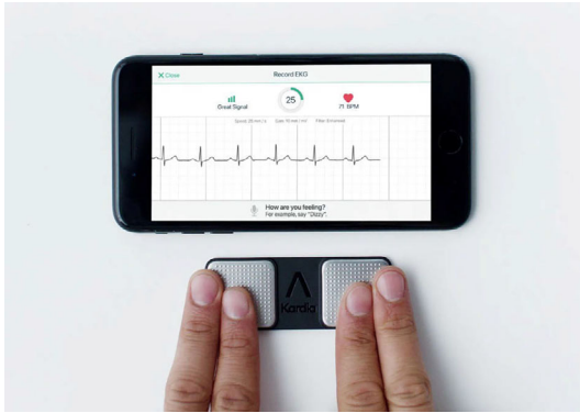
Figure 6. Personal ECG monitoring using a smartphone for Android or iPhone (Kardia Mobile®; AliveCor, Mountain View, USA). Image: KMobile-Demo_Moment.jpg. https://www.alivecor.com . Accessed June 12, 2020. Used with the permission of AliveCor.
