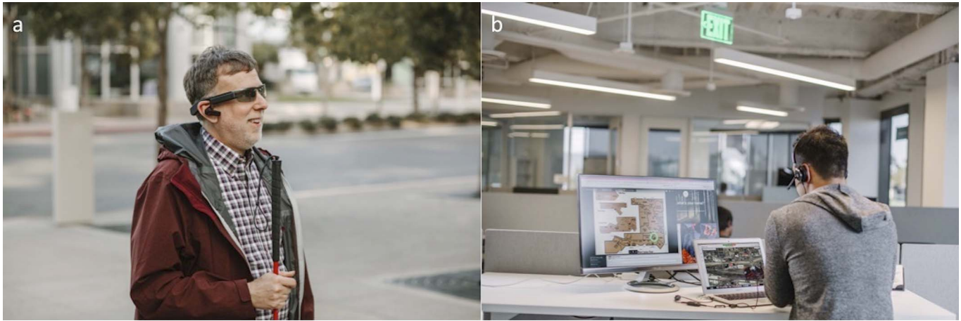
Figure 1. (a) Severely visually impaired individual using Aira with livestreaming to (b) agent with module consisting of the device's video view and applications that assist with task coordination. Pictures courtesy of Aira.
