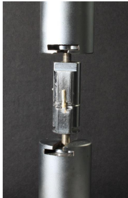
Figure 3. After obtaining 1 mm × 1 mm beam-shaped sticks by longitudinally sectioning teeth using Isomet saw, each stick was glued with cyanoacrylate adhesive to specifically designed metal plates and placed in universal testing machine. Afterward, tensile load was applied to each beam at a crosshead speed of 0.5 mm/min until it fractured.
